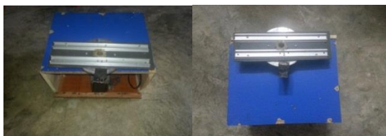
Fig.2: Foundation of the solar tracker
